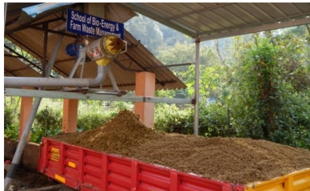
Installed dung-dewatering machine at ILFC Pookode.3 tonnes per hour dung-dewatering machine at ILFC, Pookode
