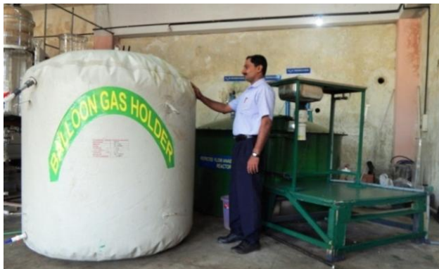
Restricted flow two stage bio-gas plant
